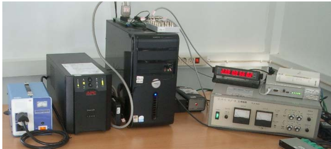
Transformer, UPS, PC, and back-end receiver (from left to right)
